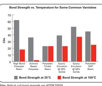
Note: Helical coil bond strength per ASTM D2519.
